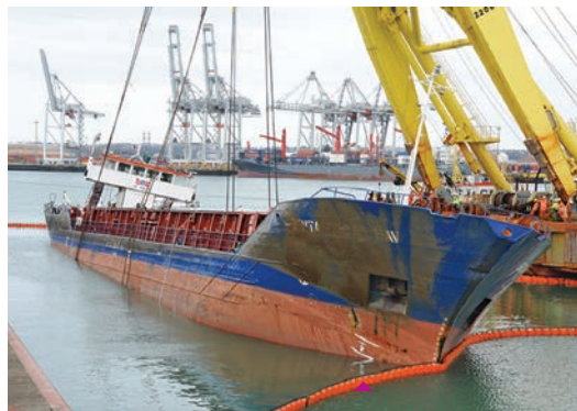
▲ Britannica Hav is righted in the port of Le Havre Image: Eric Hourii
