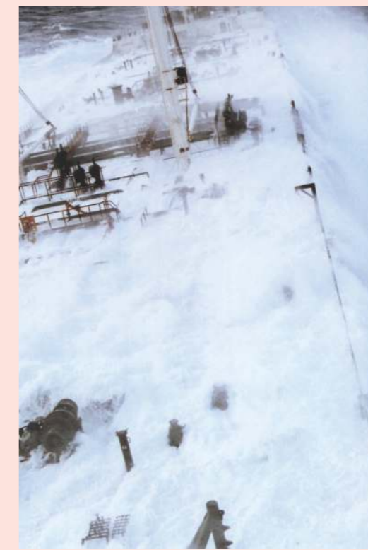
▲ The dangers of parametric rolling in severe conditions has recently been highlighted in a UK Marine Investigation Branch (MAIB) report on the collapse of three container bays and loss of 137 containers from the CMA CGM G. Washington Image: MAIB
