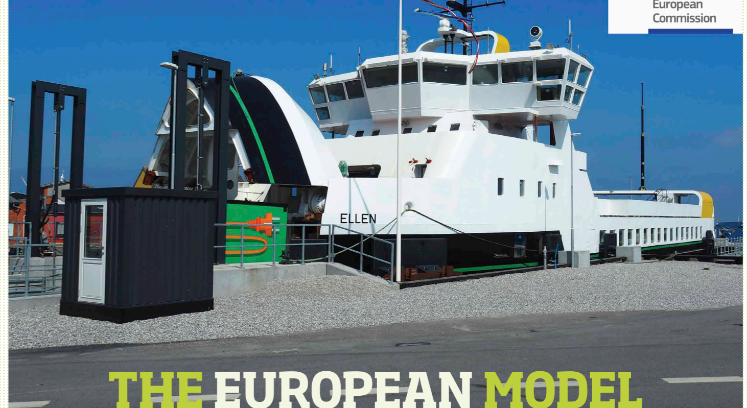
The battery-powered Danish island ferry Ellen, being charge at berth Image: E-ferry project
